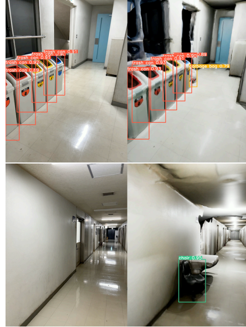
Fig. 4: Successful detection of the removal of objects: a garbage bag in the upper case and a chair in the lower case. The left image is captured by an actual camera while the right one is rendered in Unreal Engine 5.
