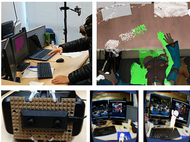
Figure 3: A captured (top left) and segmented (top right) pet stroking action. An avatar representing the user’s body is overlaid for reference. Image of the video-see through Oculus Rift DK2 (with detachable stereo cameras, bottom left), and two examples of actions and responses from the virtual pet from the view of the Rift, including begging and playful jumping (bottom middle and right).
